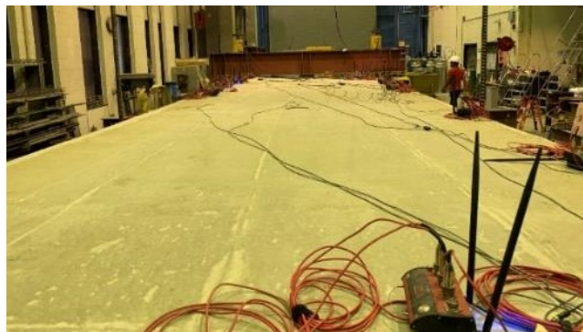
Figure 132. Test Run #45 Failure 3 setup (load at Loc. 10)
