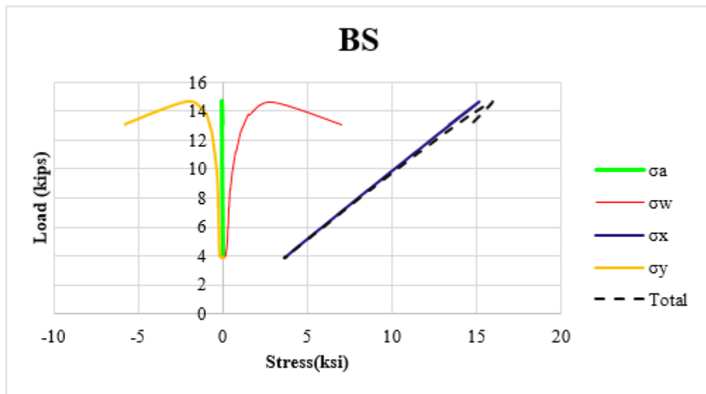
Figure 52. Stress components, Loc. 3 BS, Test Run #1
